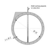
Shut-off damper with blade actuator attached.
