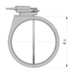
Shut-off damper with manually operation.
